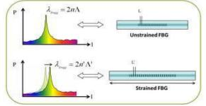
Fig.2 : Fibre Bragg Grating principle[11] Source:http://www.fbgs.com/technology/fbg-principle
