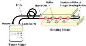
Fig. 4: Fibre optic MicrobendingSensor [2][11] Source: http://www.mdpi.com/1424-8220/10/11/10198
